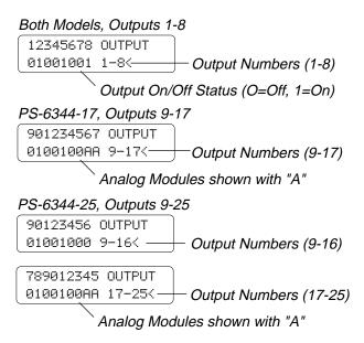
If any output positions have been programmed as analog outputs, the On/Off status will show "A" instead of "0" or "1."
