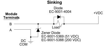
Most applications will not need the diodes shown above. However, highly inductive DC loads may damage modules by generating voltage spikes when switched off. Suppress these voltage spikes using one of these two methods:
