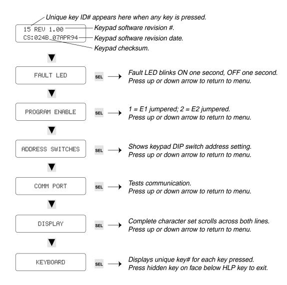
Figure 40—Keypad Communications Port Test Setup
