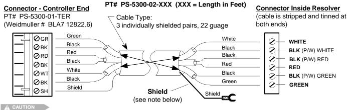
**Shielding Note:** This type of resolver cable will have a spade lug connected to the shield at the resolver end. The lug should be attached to the grounding stud on the cover plate of the resolver. In some installations, it may be advisable to disconnect the lug to prevent ground loops through the cable shield. Consult Electro Cam if electrical noise problems are suspected.
