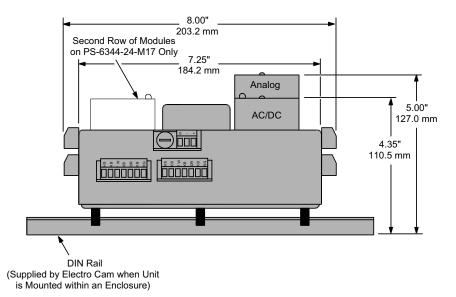
Figure 5—PS-6344-24-M17 Terminals & Components
