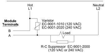
Most applications will not need the varistor or R-C suppressor shown above. However, when other switching devices are in series or parallel with the AC module, voltage spikes may damage the module. Use one of the following two methods to suppress voltage spikes.
